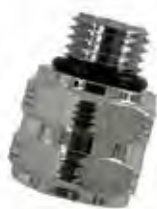
Adapter Male 7/16-20 to Female 3/8-24 Part No: EDG-AD-06 Hose to 1st Stage
